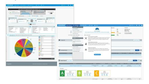
CyberFlood is a powerful, easy-to-use test solution that generates thousands of different realistic application traffic scenarios and attacks to test the performance, scalability and security of today's application-aware network infrastructures. Unlike other test solutions, CyberFlood generates real high-performance user applications based on actual application scenarios for realistic security, load and functional testing.
